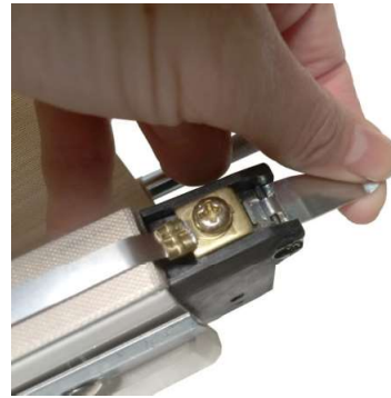
Figure 6. Lift latch on heating block to screw element in place.
