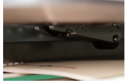
Wire-O® closing area with auto-centering of bound document
