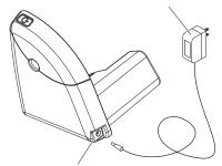
**Power Jack** - connect the power lead from the power adapter to this jack.
