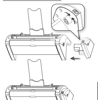
Connect the **Driving Shaft** on the **Power Pack** to the side gear of the **CardMac** firmly. If necessary, rotate the **Driving Shaft** slightly for proper alignment.
