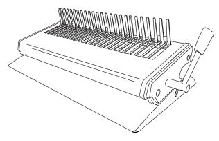
Place pre-selected comb behind Comb Binding Fingers. The opening side of comb should be on top. <u>See Picture 1</u>
