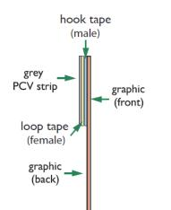
4. Add 0.63" (16mm) hook tape (male) to the top of the new graphic panel and apply the existing grey PVC strip.
