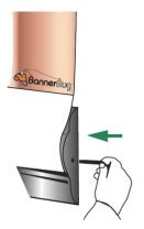
Release the graphic panel completely from the system to expose the PVC tongue and graphic join. Place the pin into the side of the unit when the hole on the roller lines up with the hole in the end cap.
