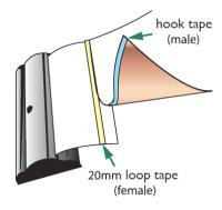
2. Carefully remove the existing graphic panel from the PVC tongue. Add 0.78" (20mm) hook tape (male) to the base of the new graphic panel and then place in the same position.
