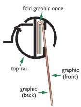
5. Fold the top of the new graphic backwards once and then slide into the top rail.
