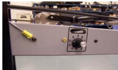
2. Attach the opposite end of the antistatic kit to the inside of the non-operator side frame using the magnet:
