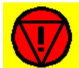
This indicates the emergency stop button is triggered and needs to be pulled to reset.
