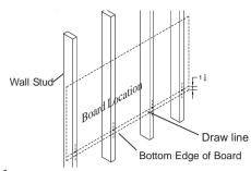
1 Determine board location. Measure from floor to the bottom edge of board. Mark with pencil line the corner location. Measure up from bottom edge of board 1-1/4" and draw line as shown. Locate stud near each end of board and drill pilot holes along line using 1/8" drill bit. See diagram below.
