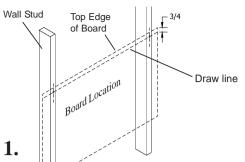
Determine board location. Measure from floor to the top edge of board. Mark with pencil line the corner location. Measure down from top edge of board 3/4", and draw line as shown. Locate stud near each end of board and drill pilot hole along line
