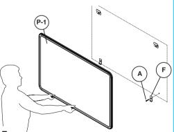
Secure 2 bottom brackets (F) to the wall using 2 long screws (A) as shown. Hang board on the Z-Hangers (E).
