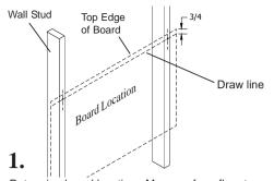
Determine board location. Measure from floor to the top edge of board. Mark with pencil line the corner location. Measure down from top edge of board 3/4", and draw line as shown. Locate stud near each end of board and drill pilot hole along line using 1/8" drill bit.
