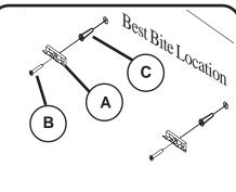
2.Install two Screw Anchors(C) and two Mounting Brackets(A) using two Screws (B).
