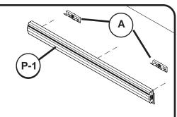
**3.** Snap the Best-Bite (P1) over the Plastic Bracket (A) as shown in Illustration #3.
