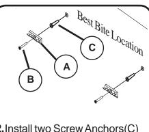
2.Install two Screw Anchors(C) and two Mounting Brackets(A) using two Screws (B).
