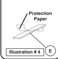
Wipe off the back of Best-Bite (P-1) to remove all particles. Place the tape's peeled sides on to the back of the unit in even spaces, and remove the other protection paper from the Double
