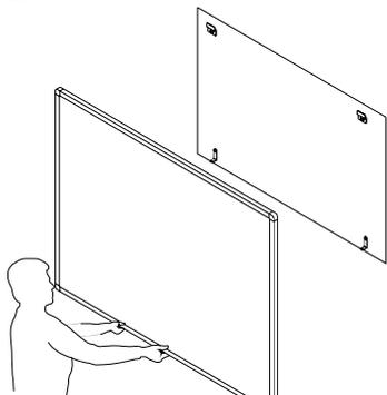
Secure 2 bottom brackets to the wall using 2 long screws as shown. Hang board on the Z-Hangers using the Hanging brackets mounted on the back of the board.
