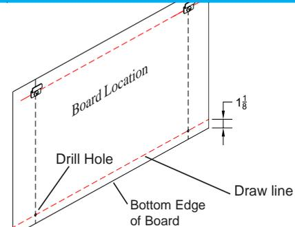
Lift and remove board from the Z-Hangers. Measure up from bottom line of board 1-1/8", and draw line as shown. Locate stud near each end of board and drill pilot hole along line using 1/16" drill bit.
