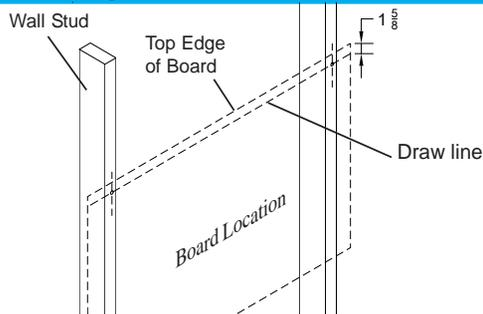
Determine board location. Measure from floor to the top edge of board. Mark with pencil line the corner location. Measure down from top edge of board 1-5/8", and draw line as shown. Locate stud near each end of board and drill pilot hole along line using 1/16" drill bit.
