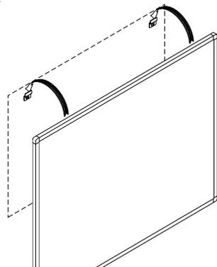
Hang board on the Z-Hangers using the Hanging brackets mounted on the back of the board. Draw line along bottom edge of board.
