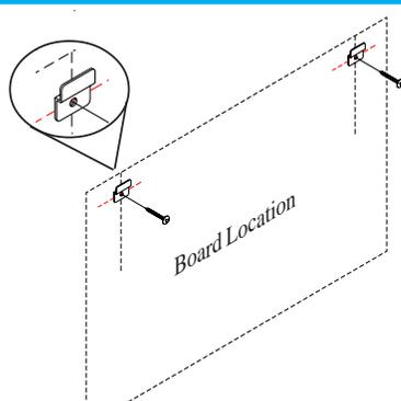
Attach 2 Z-Hangers using 2 Long Screws as shown
