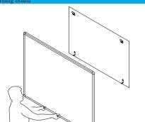
Secure 2 bottom brackets to the wall using 2 long screws as shown.
