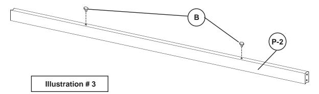
5.) Slide the Crossbrace (P2), with Bumpers (B) facing up, in between the Posts (P3) and up to the bottom of Board (P1). Line up the the Crossbrace's (P2) mount holes with the holes in the Posts (P3) and secure using two Screws (A2) on each side as shown in Illustration #4.
