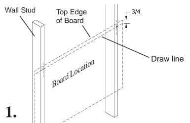
Determine board location. Measure from floor to the top edge of board. Mark with pencil line the corner location. Measure down from top edge of board 3/4", and draw line as shown. Locate stud near each end of board and drill pilot hole along line
