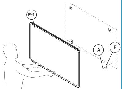
Secure 2 bottom brackets (F) to the wall using 2 long screws (A) as shown. Hang board on the Z-Hangers (E).
