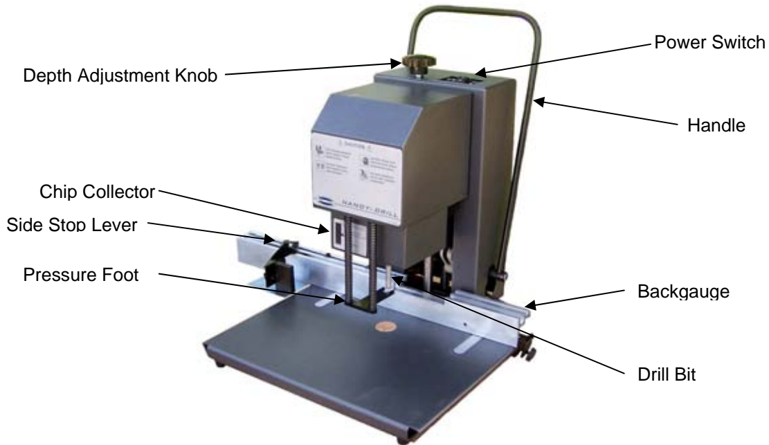
Figure – Machine Controls
