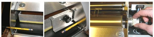
Place a pencil under the right and left carriage walls to keep the roller up out of the adhesive. Move the wiper blade as close as possible to the coating roller. Using the gear on the right, turn the coating roller a couple of revolutions to remove excess adhesive from the roller. Turn off the power and unplug the cord so the adhesive solidifies.
