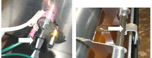
When you swivel the coating roller down into the tray, be sure the wiring goes through the square slot in the aluminum wall so the wall does not crush the wiring. Also make sure the rod support is in place. Plug it in and turn on the power. After the Maxit warms up, reset the wiper blade for the proper coating.
