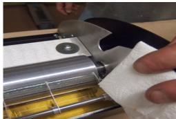
Using insulation, hold the back of the aluminum carriage walls and swivel up the assembly out of the adhesive towards the front.
