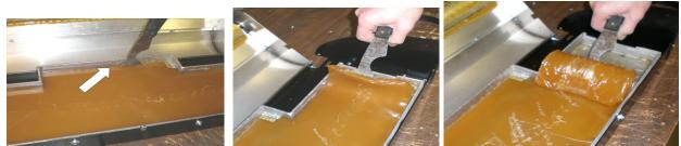
Take a putty knife and insert it along the front of the tray to separate the adhesive from the front side of the tray where there is less heat. Take the putty knife and insert it under one end of the adhesive and roll the adhesive towards the middle of the tray.
