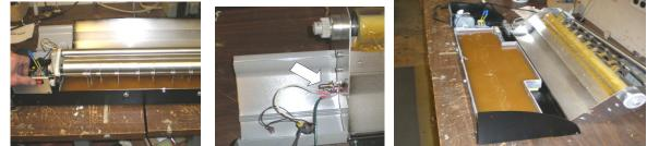
Turn the Maxit around so the back is facing the front of the table. (When you plug in the Maxit be very careful not to touch the live thermostat on the left) Plug in the Maxit and turn on the power for exactly 3 minutes, **then unplug the cord**. Swivel the coating roller away from the tray.
