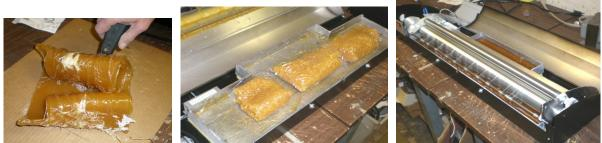
Place the adhesive on a newspaper or board. The tray does not have to be perfectly clean, so you can leave in some residue. Refill the tray with the adhesive. Swivel the coating roller back down into the tray.
