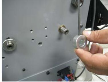
Next, remove the non-operator side cover. Loosen the belt tensioner idler pulley bracket. You do not need to remove these as loosening them will allow enough movement to free the belt. Remove the belt. Walk the motor belt off the inner pulley. If it is too difficult to walk off you could loosen the motor and pull it up as it is mounted in slots.
