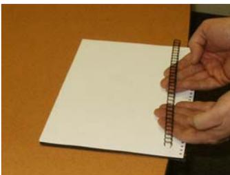
Put punched sheets together into a complete book (also take out the bottom page and place it on the top- see below) with punched edge facing you. Prepare a wire element.
