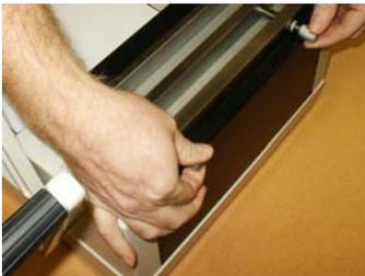
Set closing mechanism measurements, test wire closure, and adjust to satisfactory close.
