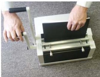
Hold book together and lift with binding edge (and binding wire) pointed downward. Wire should rest easily and naturally in punched holes. Lower the binding edge (and wire) into wire closure mechanism, placing wire down onto steel surface, and close binding handle to close wire. (TitanWire machine showed)
