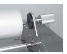
Load the mandrel on the laminator by inserting the slot end of the mandrel into the tensioner on the right side and then lowering the hanger end into the bracket on the left side.
