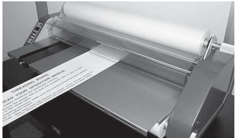
Start the motor by pressing the “Fwd” button. Feed the threading board and film in between the heat shoes. This will pull the film through the rollers until it comes out the back of the laminator.
