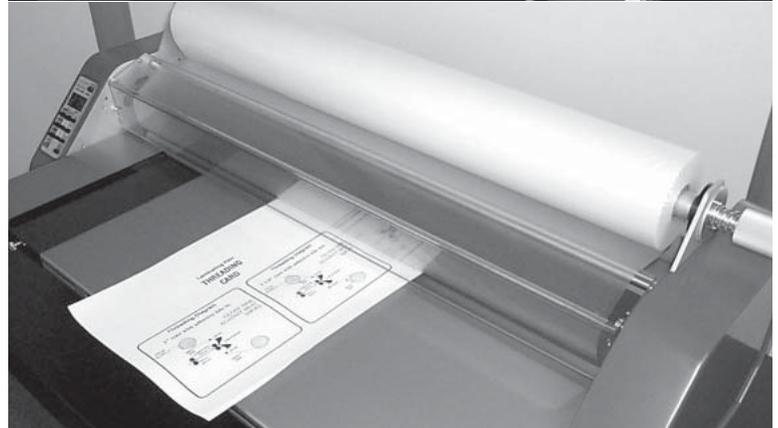
Slide the top and bottom film rolls from side to side on the mandrels so that the film is perfectly aligned top and bottom (Note: overlap will cause the film to deposit residue on the heat shoes and rollers, so this procedure is critical). Replace feed tray and heat guard.
