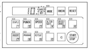
(3) Press the MODE key to change the display beside the Counter from SHEET to SET, then input the number of batches.
