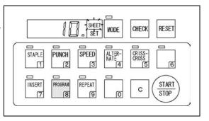
(3) Press the MODE key to change the display beside the Counter from SHEET to SET, then input the number of batches.
