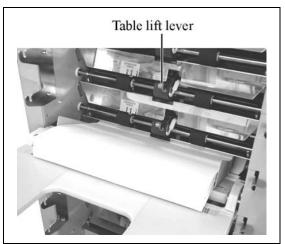
(2) Insert the right side shaft of the paper feed table in the hole on the side opposite the collator operation side, and mount the left shaft on the plate with the U-shape slot.
