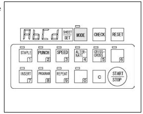
(3) Press the key responding to A to d for three seconds and memorize the data.
