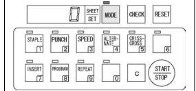
(2) Press the PROGRAM/8 key for three seconds; the Counter lamp will flash. Then, input the number of sets to be collated.
