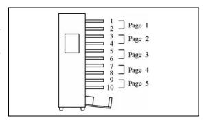
• Loading paper with the printed side down in Alternate mode.
