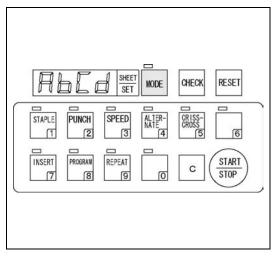
(3) Press the key to respond to A to d for three seconds and memorize the data.
