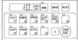
(2) Press the MODE key to switch to Function mode.
