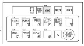
(2)Press the SPEED/3 key to change speed. Each time the MODE key and SPEED key are pressed,
