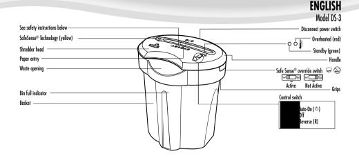
🕮 Breakthrough Safety Technology! SafeSense® stops shredding when hands are too close to the opening.
