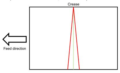
3. To adjust crease skew, loosen the crease adjustment knob by rotating it counterclockwise.
