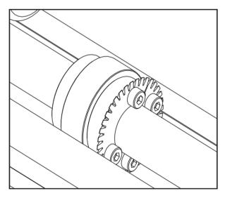
5. Using a 2 mm hex key loosen one of the drive hubs [E] and slide it away from any obstructing drive wheels or hubs in order to mount the anvil.
