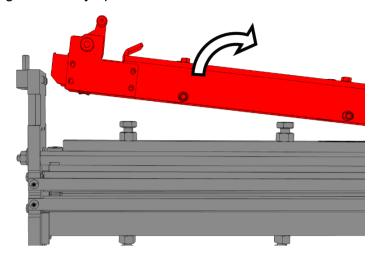
5. Pull the blade set upwards to remove it.
