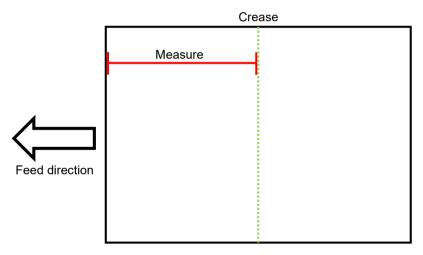
3. If the measurement is not within the machine tolerance ( $\pm$  0.25 mm /  $\pm$  0.001") contact your Dealer to perform machine re-calibration.
