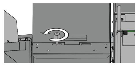
9. Move the knob slightly, either to the left or to the right depending on the direction of the crease skew.
