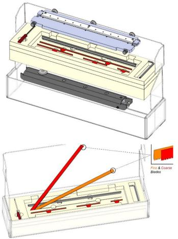
This machine can perforate across the full width of sheets with the optional cross perforation kit. V@Ápatent pending "radius rock-perf motion" together with precision perforation software requires less force compared to a straight downward stroke. The rocking motion will give a superior and more even result over the full width of the sheet. This ensures a higher precision perforation on heavier stock.
