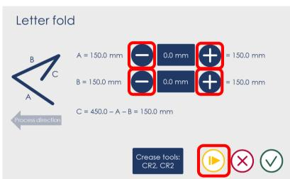
3.1. Each pattern has an adjustment screen that allows making small corrections to crease positions to achieve the desired output. Use the + / - buttons to make the adjustment and press the Proof button to run another proof sheet. When satisfied click the green tick mark.
