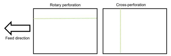
Depending on paper type and the desired finish several different perforation types are available with varying number of teeth per inch (TPI):
