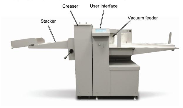
The Formax Atlas C150 is a state-of-the-art paper creasing system. Having a good crease is key to producing perfect folded jobs such as brochures, leaflets and invitations. Creasing ensures the fold is square and the printed image does not crack when folding, giving the job a premium finish.
