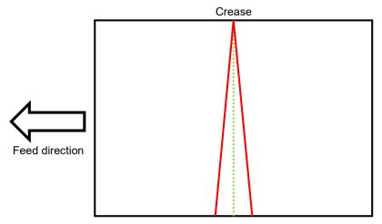
8. To adjust crease skew, loosen the crease adjustment knob by rotating it counterclockwise.
