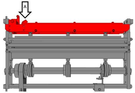
3. While pushing down, pull the Bridge Assembly towards the operator side [B]
