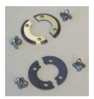
To set up rotary perforation a perforation blade and an opposing hardened anvil is necessary. This machine comes with a single perforation blade and an anvil. The perforation blades and anvils are split into two matching halves and are fitted to the drive wheels using the four screws supplied. Do not mix the matching pairs of blades or anvils as this will result in poor perforation.
