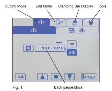
Press the Back Gauge position block (Fig. 2) on the 4. keypad to set the back gauge position for desired cut size. Press Enter.
