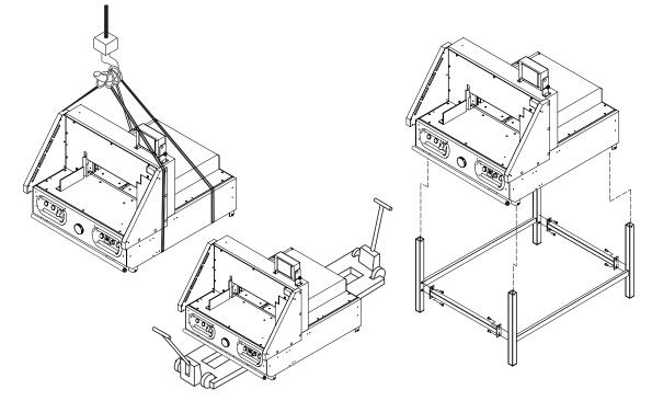
The cutter can be moved by using an overhead motorized lift, pallet jacks, or by hand. **NOTE:** Four people are required to move the cutter by hand.
