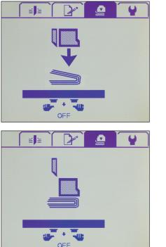
Stage 3: The clamping bar is going up when you push either of the clamp enable buttons.
