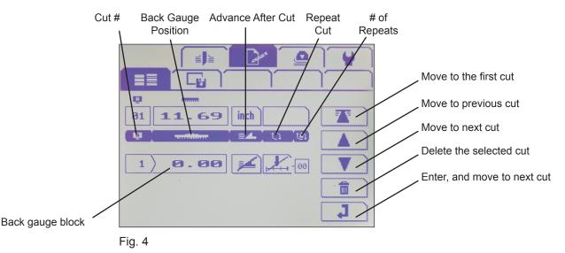
Enter position of back gauge for first cut, then press Enter.
