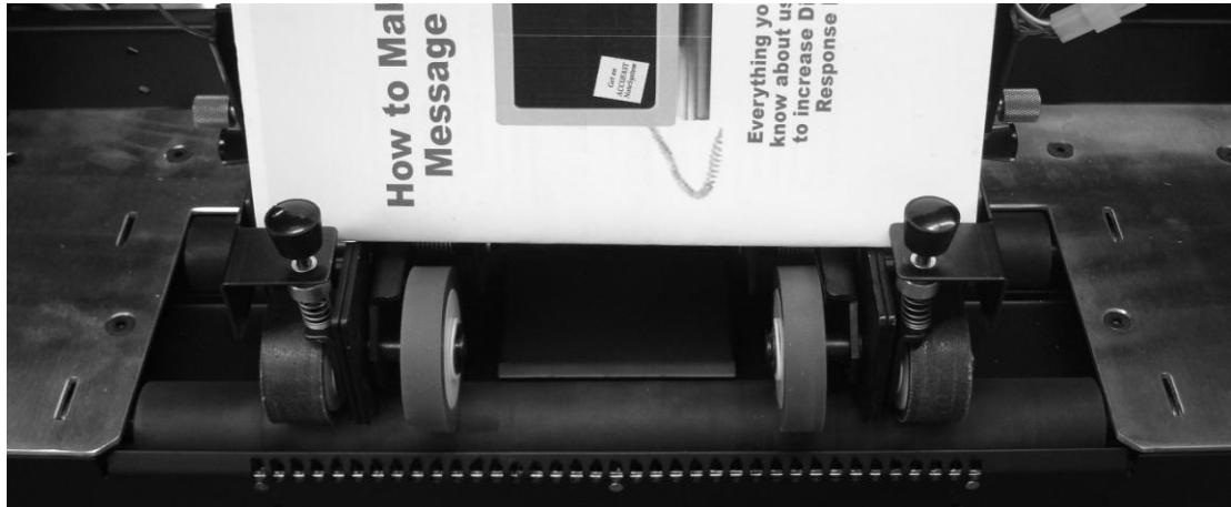
Figure 6.4 Setting the heads to match a piece on the FD 280
