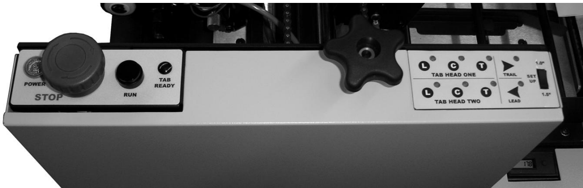
Figure 4.1 - FD 280 Operator Panel Controls
