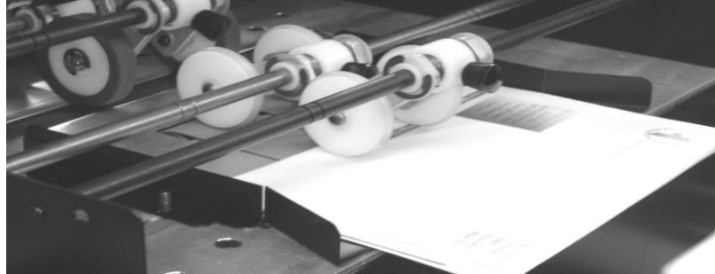
Figure 6.3 Setting up Input Guides on the FD 280
