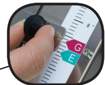
Align the fold stop notch with the matching letter.
