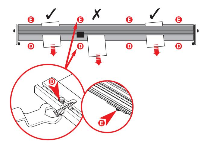
Adjust the clamping by turning the Jacking Screws "①" & "3" in the Base Fixing Brackets that are adjacent to the areas that are not clamping the paper. Turn the Jacking Screws clockwise (as you look down on them) using the wrench supplied, turn both the front and rear Jacking Screw by the same amount (to keep the Bracket level) until the paper is gripped. You may find that two or three adjacent Brackets need adjusting if you have a wide area that does not clamp.
