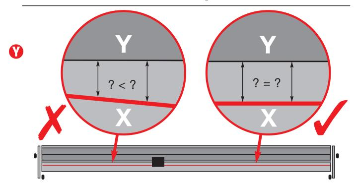
**Adjust** the straightness of the Base by adjusting the front "A" and rear "B" grub screws in the Base Fixing Brackets:
