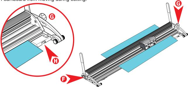
NOTE: If you are cutting a small piece of board place it at right hand end of the Cutter Bar against the Material Stop and place scraps of the same thickness material under the remaining bar to support it and prevent sagging.
