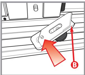
Before tightening the clamping screw the blade depth can be adjusted by sliding the adjustment knob up or down to retract or extend the blade. It is good practice to set the depth so that the minimum amount of blade is exposed to just cut through the material, it takes much less effort and produces a better cut.
