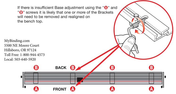
Place two of the long wood screws "A" in the front holes of the Fixed Arms and partially insert them into the bench surface but do not tighten. Loosen, by one full turn anti-clockwise, the four hexagon socket screws "B" joining the Fixed Arms to the Base. Fully insert the two wood screws "A".
