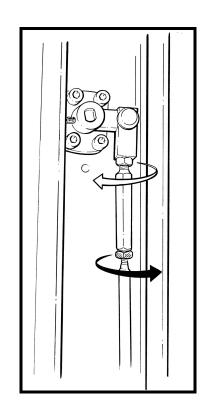
The 'adjuster' is the hexagonal bar between the two nuts, by turning it with the wrench it alters the clamps alignment with the back of the machine.
