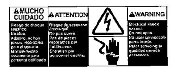
This means an electrical shock hazard exists if covers, enclosures or guards are removed and internal parts become accessible. ALWAYS refer servicing to gualified GBC service personnel.
