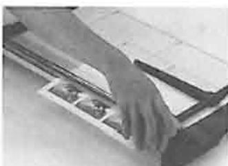
3. Press and slide blade to cut media. Slide cutting head to the far left or right to place in locked position.
