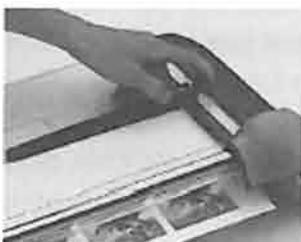
2. Adjust the media guide to the proper position. Can be removed for larger applications.
