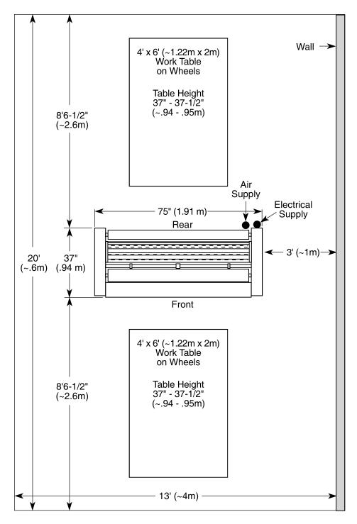
Figure 2-1: Laminator Space Requirements
