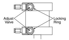
Figure 4-5: Adjusting the Air Cylinder Flow Controls
