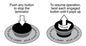
Figure 3-1: Using the Emergency Stop Buttons
