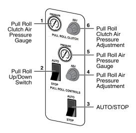
Figure 3-4: Rear Control Panel
