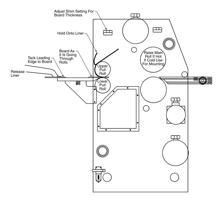
Two Pass Cold Mount/Cold Laminate (First Pass)
