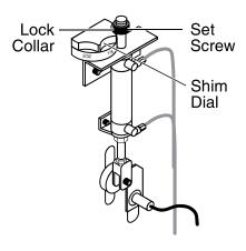
Figure 4-2: Adjusting the Pull Roll Nip
