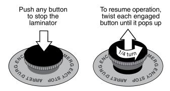
Figure 1-1: Using the Emergency Stop Buttons
