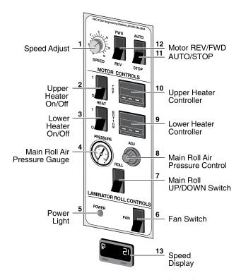
Figure 3-3: Front Control Panel
