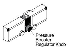
Figure 4-3: Pressure Booster Adjustment
