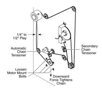
Figure 4-4: Adjusting the Chain Tension
