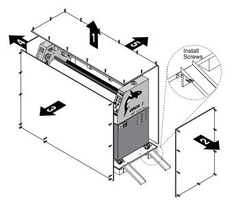
Figure 2-2: Removing the Crate
