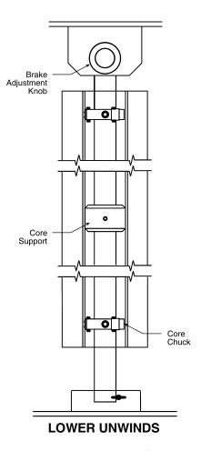
Figure 3-5: Brake Configuration
