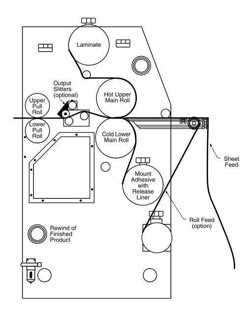
Two Pass Hot Laminate/Cold Mount (Second Pass)
