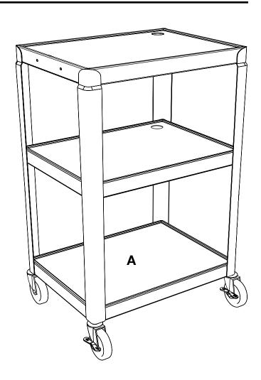
Position the cart frame A so that the caster holes are facing up. Insert caster **B** into the caster holes on the bottom of A. Use a mallet to set the casters properly.
