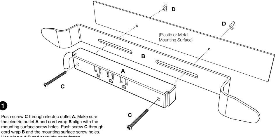
Use wing nut **D** and screwdriver to fasten.
