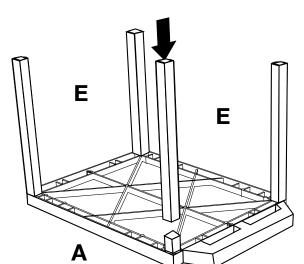
Slide and align runner **H** & **G** onto the legs and tighten screw **N** with a screwdriver.
