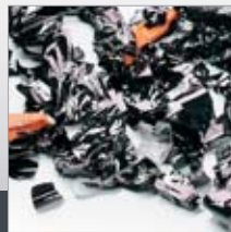
Particles of shredded magnetic tapes, credit cards and customer cards Cutting size 20 x 40–50 (1,000 mm 2 )
