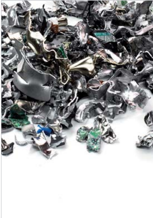
Particles of shredded hard drives Cutting size 10 x 25–30 (300 mm 2 )
