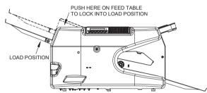
Load the paper into the Feed Table, making sure that the paper is fully within the folder, and that the leading edge of the stack is resting against the face indicated below. Once the Feed Table has been loaded with paper, the Feed Table must be unlocked, allowing the Feed Table to return to the raised position. To unlock the Feed Table, press the Feed Table Release (see illustration below).
