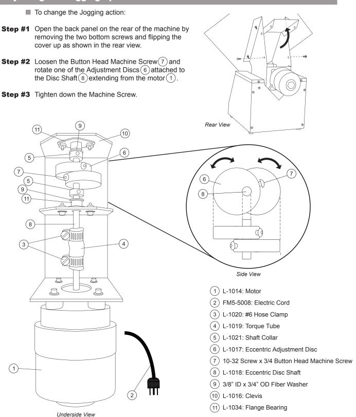
**Note:** When the screws are located opposite each other on the shaft, the minimum action is obtained. When the screws are located on the same side of the shaft, the maximum action is obtained. Normal action is obtained when the screws are 80° to 90° apart.
