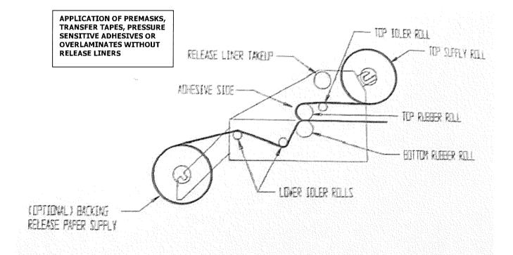
MIE: The operator rust use a backing paper either from a supply roll or in sheets to prevent achesive from adverting to the machine
