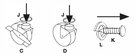
Hold Caster **C** (with Ring Seater **J** on it) up in the bottom of Tubular Frame **B**. Insert Screw **K** (with Spring Washer **L** on it) into the frame and using Hex Wrench **M**, secure the Caster. Do the same with all of the Casters. **Note:** Both Caster **C** pieces should be attached on the same side as shown. **Note:** Once Casters are attached, go back and tighten all Screws until secure.
