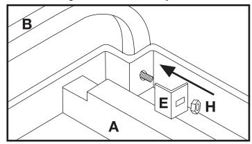
Attach the 2 remaing Molded Tray **A** pieces onto the Tubular Frame **B** as Step 1. Assemble the second Tubular Frame **B** onto the other side of the Molded Tray **A** pieces.
