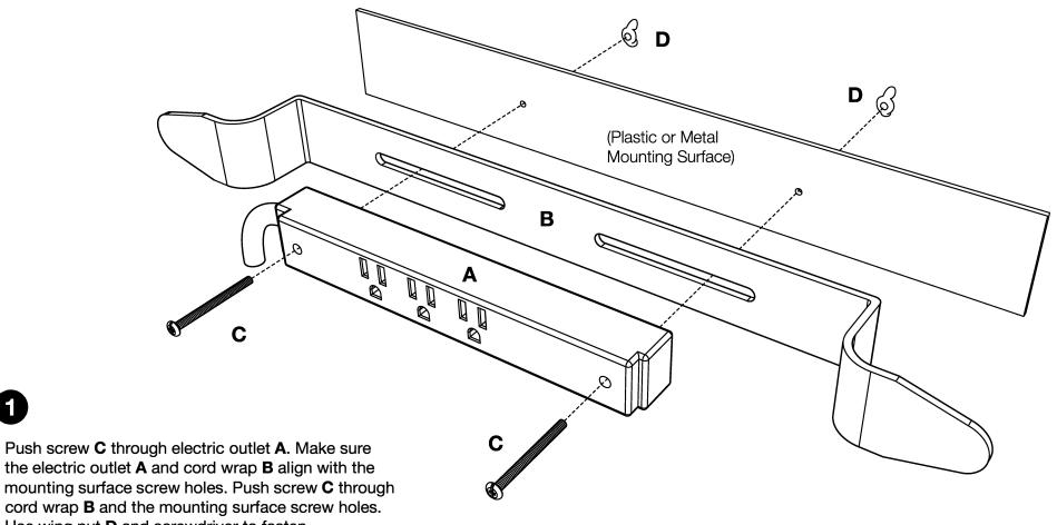
cord wrap **B** and the mounting surface screw holes. Use wing nut **D** and screwdriver to fasten.
