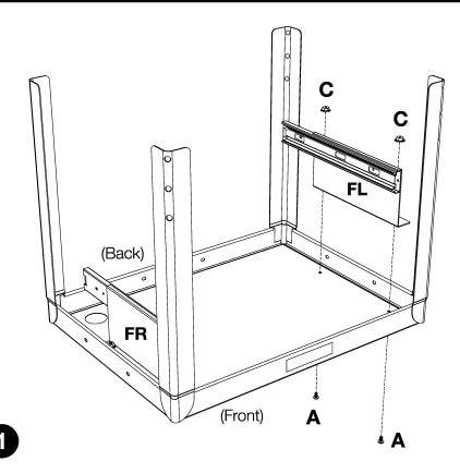
Take the top shelf of your metal cart and lay it flat. Collect parts: **FL**, **FR**, **A** & **C**. Push Screw **A** through the hole at the top of the shelf. Lay bracket **FL** & **FR** on top of screw **A**. Take nut **C** and fasten with a screwdriver and pliers, do not tighten fully until shelf is attached.
