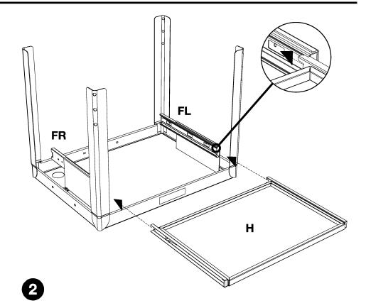
Collect parts: **H.** Align the pullout shelf **H** runner so that the runner snaps into place into the **FL** & **FR** brackets. Pull the shelf out to make sure it is fully seated. Tighten screws **A** and nut **C**. Pullout keyboard shelf assembly is now complete.
