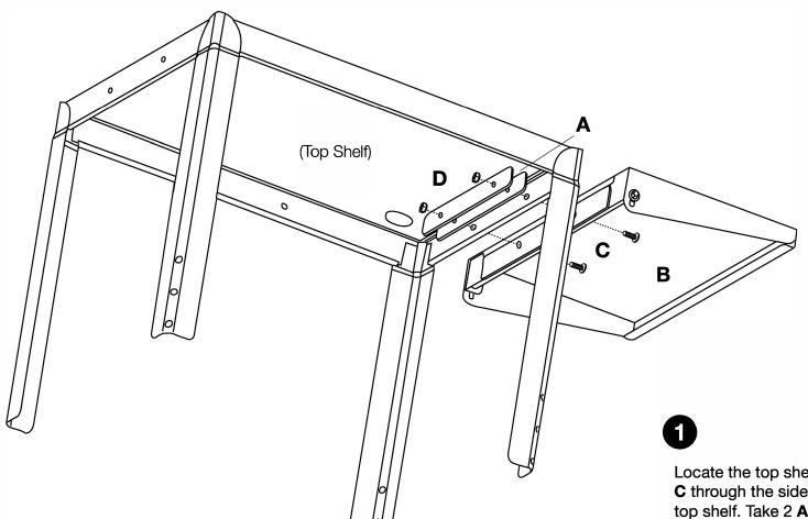
Locate the top shelf of your metal cart. Push screw C through the side holes of drop shelf B and the top shelf. Take 2 A brackets and push them through screw C. Take nut D and fasten with a screwdriver and pliers. Repeat this on the other side.
