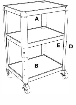
Position the bottom shelf **B** so that the caster holes are facing up. Insert caster **C** into the caster holes on the bottom of shelf **B**. Use a mallet to set the casters properly.
