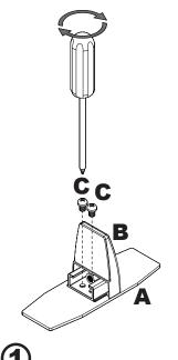
Attach B to A with Screws C
