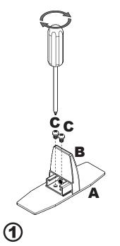
Attach B to A with Screws C
