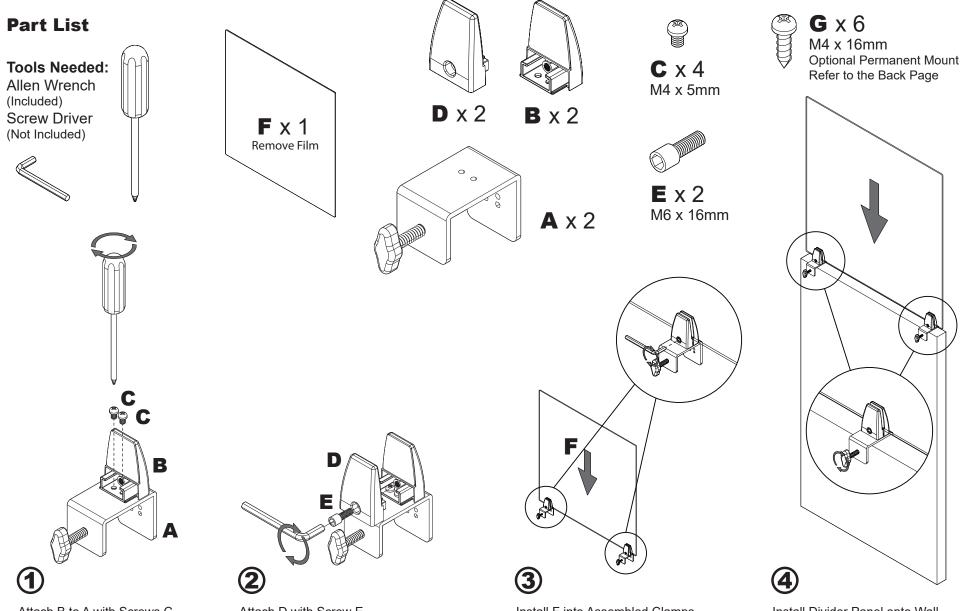
Attach B to A with Screws C
