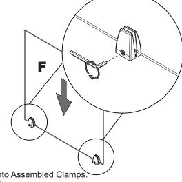
Install F into Assembled Clamps.
