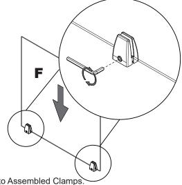
Install F into Assembled Clamps.
