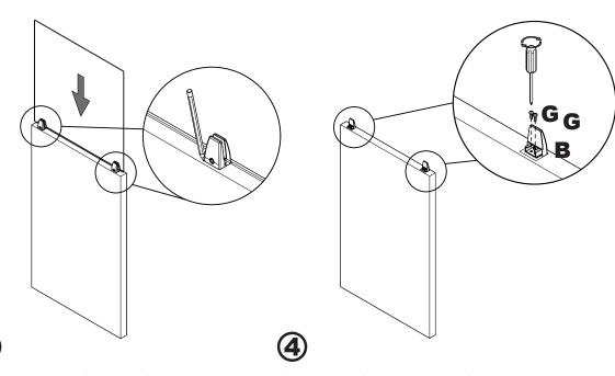
With Assistance - Place the Panel Assembly on the Wall and Outline the Clamps with a Pencil.
